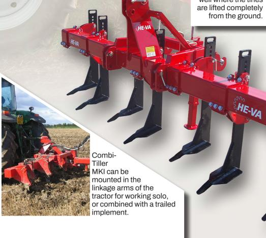
The quick couplings allow the HE-VA Combi-Tiller MKI to be built together with another three-point mounted implement, for example the HE-VA Disc-Roller.
