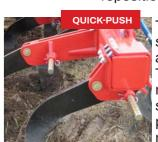
The Quick-Push shear bolt breaks if a tine hits a stone. Then the R-clip is removed and the shear bolt is easily pushed forward into new position
