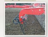
For cultivation aimed at creating a stale seedbed, a pre-mounted tine harrow with 16 mm tines can be used to ensure surface soil
