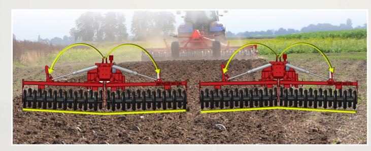
Its hydraulic folding mechanism is linked to two accumulators and a hydraulic pressure gauge. The operator can distribute pressure evenly across the working width for consistent cultivation on uneven ground. The accumulators act as an oil buffer, while hydraulic cylinders extend or retract to allow the disc cultivator to follow surface contours.
