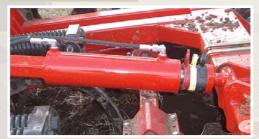
On all models the working depth is adjusted hydraulically from the cabin with the possibility of fixed stop via the distance clips.
