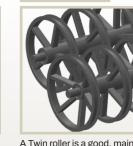
A Twin roller is a good, maintenance free solution, as the rollers clean each other while operating. The Twin roller with U-profile ensures good soil-
