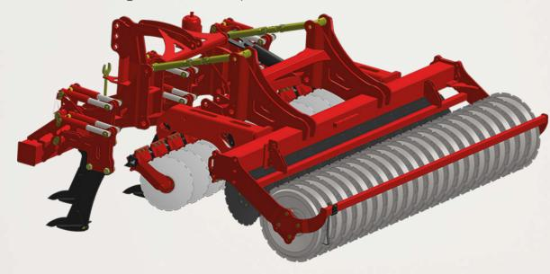
The Combi-Disc provides versatility by being able to perform a number of different jobs from primary cultivation to secondary cultivation and from subsoiling to shallow disc cultivating. It can be used as a subsoiler with the discs lifted out of work, a disc cultivator with the legs lifted up, or as a complete one pass cultivator – all of this without leaving the tractor seat allowing for minute changes to settings whilst working in the field.
