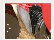
Trailed machines can be fitted with front discs in line with the subsoiling tines to reduce surface soil disturbance.
