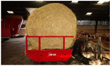
The machine is equipped with two integrated spears. These can be used to handle and load the bale onto the unwind table without the driver having to leave the tractor seat. The spears are then backed into engagement with the machine whereby the transmission is automatically engaged.
