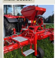
Grass-Combi can be equipped with HEVA Multi-Seeder for re-sowing.
