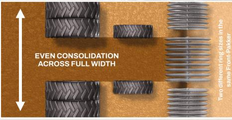
The 700 mm and 800 mm rings give good allround pressing on light, medium and heavy soils and yet have a low rolling resistance due to their weight to diameter ratio and the shoulder profile.
