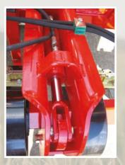
All machines that incorporate a Spring-Board have hydraulic adjustment of the working depth, so that the aggressiveness can be adjusted on the move or the Spring-Board lifted out of work completely if the conditions dictate.
