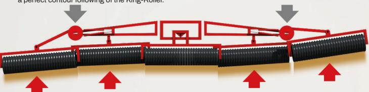
HE-VA King-Roller is available with 10 different ring types, including the big 24"/620 mm Cambridge rings (20.30 m King-Roller: only 6 ring types). The rings are mounted on 60 mm special steel axles suspended in double sealed 60 mm large flange ball bearings. King-Rollers are mounted with support bearings on all sections (however not on the outer sections of the 12.30 and 15.30 m models).
