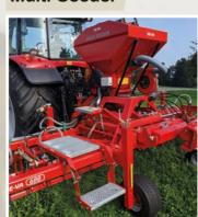
Grass-Combi can be equipped with HEVA Multi-Seeder for re-sowing.
