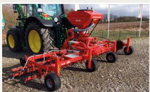
The standard mounted rear snap coupling also allows the Grass-Combi to be used in combination with a trailed roller. In this case, the HE-VA Tip-Roller is the ideal solution.
