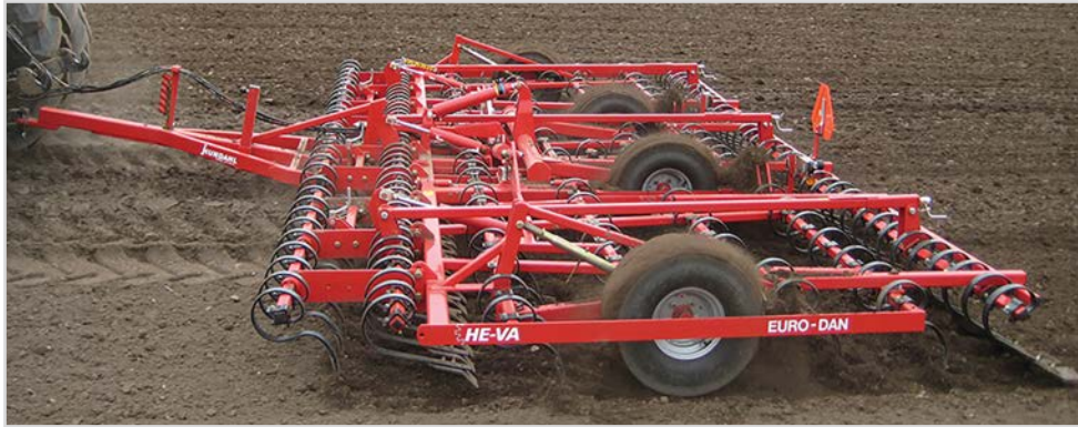
Euro-Dan Eco 8.00 m with Strong front-harrow, Spring-Board spring tine levelling bar and Spring-Board after-harrow.
