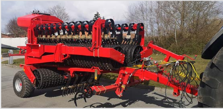
Folded Tip-Roller with Multi-Seeder, Spring-Board and wheel track eradicator.
