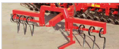
Wheel track eradicator frame for lift.
