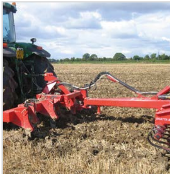
Combi-Tiller MKI with three-point linkage for combination with several lift mounted/trailed implements. E.g. bed formers for potatoes or trailed drill units.
