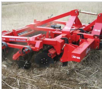
Combi-Tiller MKI with three-point linkage for combination with a lift mounted Disc-Roller Contour. Incl. 1 set of hydr. extension hoses, extension cord for lights and supporting legs f/Disc-Roller Contour.
