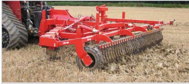
5.00 m Sub-Tiller with V-Profile rings and hydraulic automatic stone protection.
