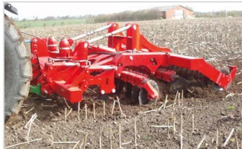
Combi-Disc with the tines in max. working depth, ensuring a soil loosening, cultivation and a consolidation.
