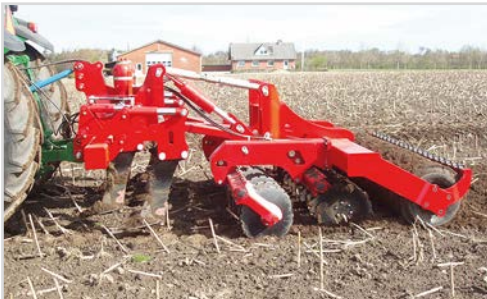
Combi-Disc with the tines lifted free from the soil, meaning that only the Disc-Roller's function is in work.
