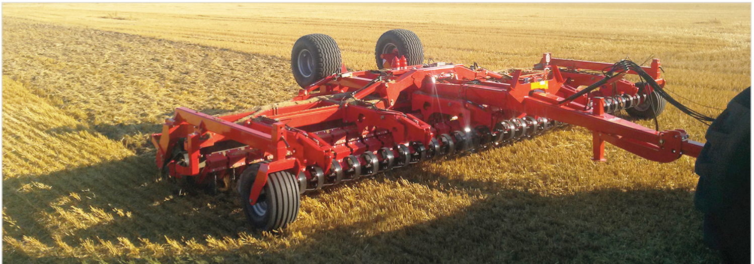
6.50 m Disc-Roller Contour with V-Profile Roller, material damper guard, pivoting support wheels and two-point pivoting crossbar.
