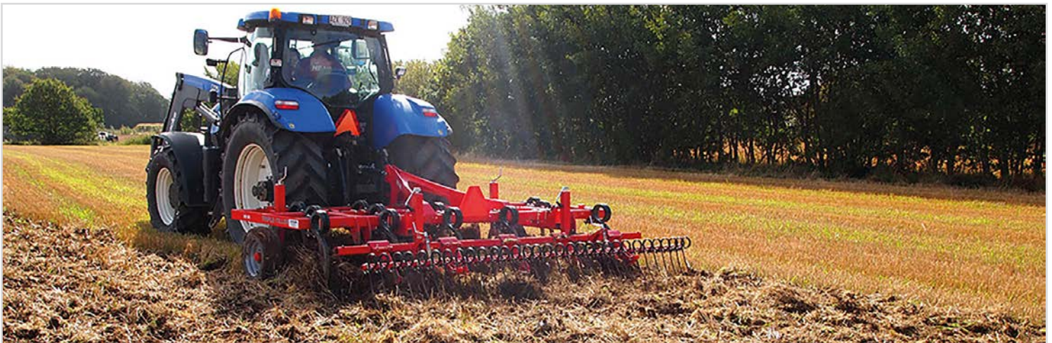
4.00 m Triple-Tiller Airy with spring tines.
