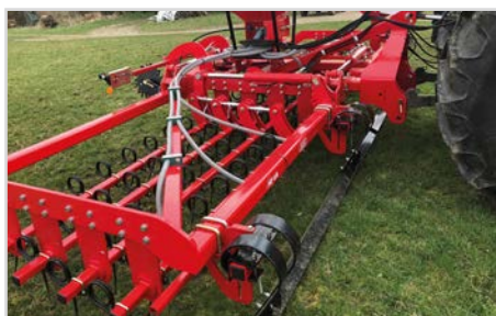
Levelling bar with spindle height adjustment.
