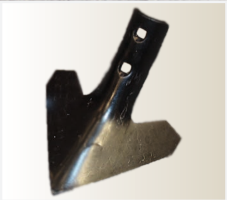
65x12 mm tines with 15 cm row spacing for a lighter harrowing to maintain the surface structure. This tine allows the harrow to be used for light stubble preparation, a full cutting of the surface is ensured with the 180x6 mm goosefoot point.
