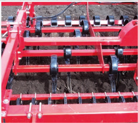
65x12 mm tines with 15 cm row spacing for a lighter harrowing to maintain the surface structure. This tine allows the harrow to be used for light stubble preparation, a full cutting of the surface is ensured with the 180x6 mm goosefoot point.
