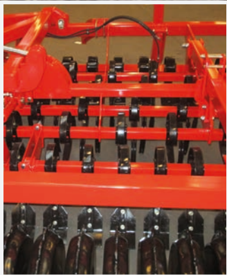
45x12 mm tines with 8.5 cm row spacing for a fine and uniform seedbed preparation.
