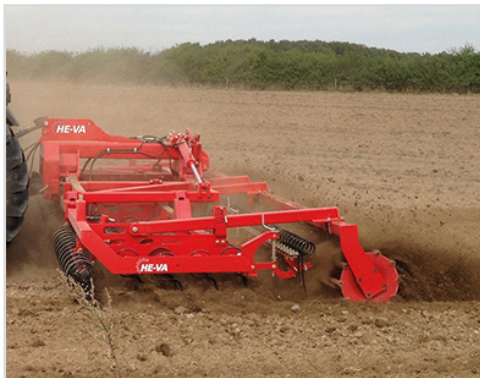
7.50 m three-point mounted Terra-Dan MKII with Square Tube Roller.
