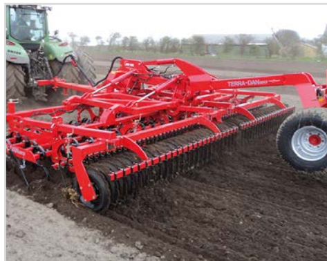
7.50 m trailed Terra-Dan MKII with V-Profile Roller.
