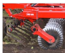
Standard disc, 610x6 mm - fine profile.
