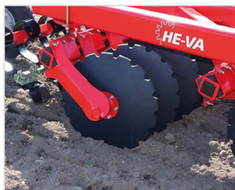
Standard disc, 610x6 mm - fine profile.
