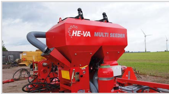
Multi-Seeder Twin 2x100-8-HY-AC 593 x 926 (1.180) mm H=935 (1.075) mm
