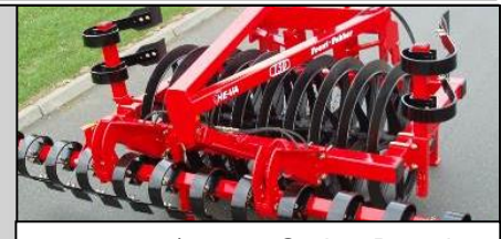
1,5 m m/4,00 m Spring-Board in transport position.
