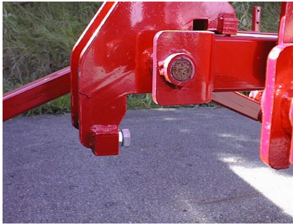
Justérbart vingestop. Adjustable stop for sideframes.
