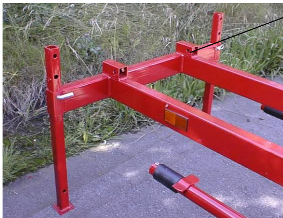
Støtteben anbringes i røret (1), inden vingerne slæes ned. The support jacks are placed in the tubes (1), before the sideframes are folded down.
