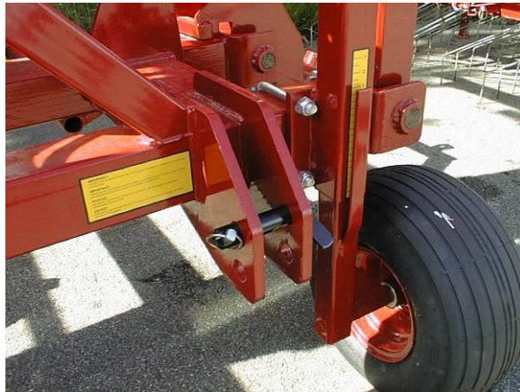
Tilkobling på 9,0 og 12,0m. Attachmentplates on 9,0 and 12,0 m.
