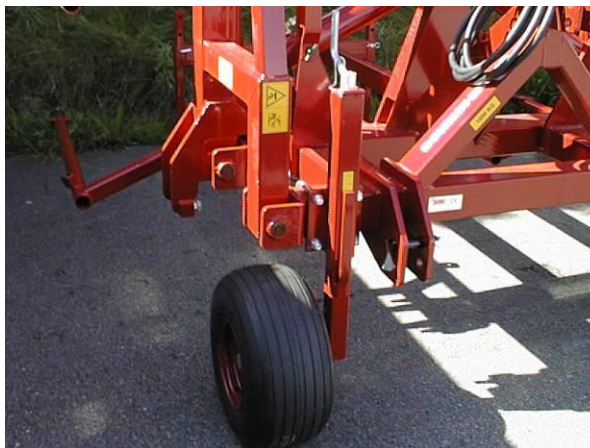
Bærehjulene justeres så harveled står vandret, husk at låse spindelen. The supportwheels has to be adjusted, so that the harrowframes are horizontal durind work. Remember to lock the spindle
