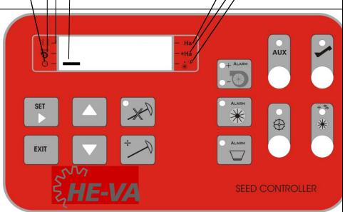
Fan alarm: If the fan rpm +/÷ is changed 10% in relation to the set alarm, a lamp will light up and an audible alarm will be activated. The sound will be disconnected by pressing this key and the lamp lights up until the desired fan rpm is re-achieved.
