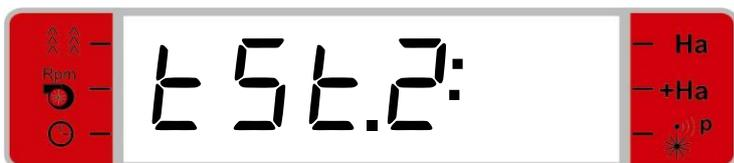
Display for test of switches (indicating "tSt.2." in the display).
