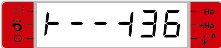
Display for setup of spray width.
