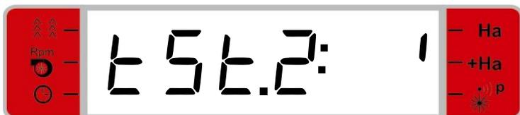
Example of test of
