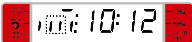
The above display shows that a half seeding width is used for the first passage, that the actuator shall be placed in the middle for symmetric tramline positioning and finally that it is not important to which side the seeder is placed in the first passage (no flashing horizontal markings in the middle/at the bottom of the display). Furthermore, it is shown that the start passage is the 10th passage in a cycle of 12.
