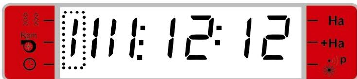
The display shows that asymmetric tramline positioning has been selected with a cycle of 12.
