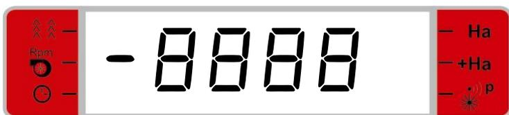
The display for indication of the blower RPM.
