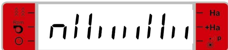
This display shows that actuator 1 shall be installed 1/4 seeding width inside from the left side. Actuator 2 shall be installed 1/4 seeding width inside from the right side. At the same time the start direction is shown at the horizontal bar in the left side. This indicates that it shall be started so that the property line of the field is to the left.
