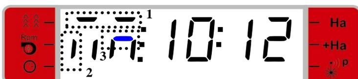
The above display shows that a full seeding width is used for the first passage (field 1), that the actuator shall be placed in the left side for asymmetric tramline positioning (field 2) and that you will start in the right side of the seeder towards the property line (field 3). Furthermore, it is shown that the start passage is the 10th passage in a cycle of 12.
