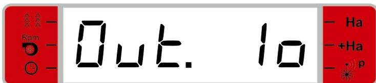
Display for test of outputs. Here output 1 is activated.
