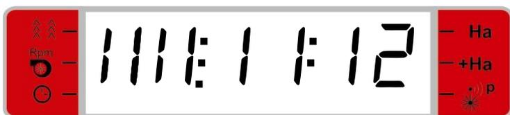
The display shows that work is being performed on the 11th passage out of 12 and therefore no tramlines are being laid (no segments are flashing).
