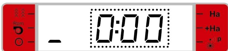
If you press the SET key for two seconds, this will imply that the reset time of operation is saved. If the time of operation should not be reset, you may press the EXIT key in order to maintain the previous value, and the Controller will then leave the edit mode and show the previous display. If you press the EXIT key again, the Controller will show the display for the tramline positioning.
