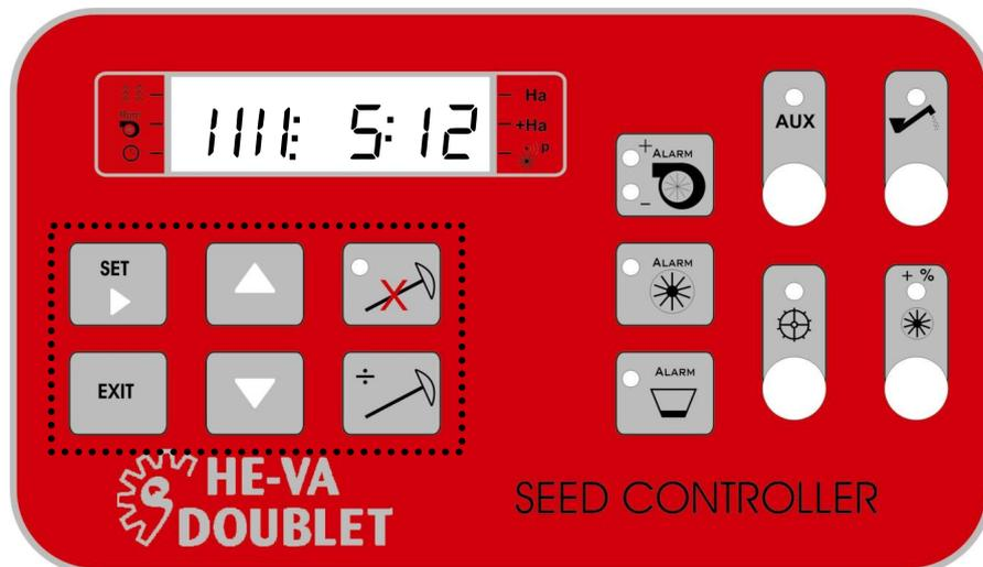
The locations of the control keys are framed in the broken line field.
