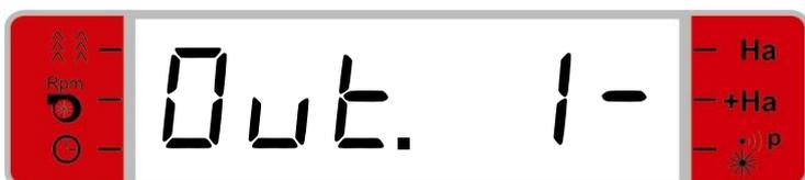
Display for test of outputs. Here output 1 is deactivated (middle segment signals deactivation).
