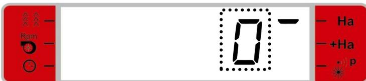
If you press the SET key for two seconds, this will imply that the reset part area is saved. If the part area should not be reset, you may press the EXIT key in order to maintain the previous value, and the Controller will then leave the edit mode and show the previous display. If you press the EXIT-key again, the Controller will show the display for the tramline positioning.
