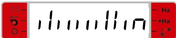
This display shows that actuator 2 shall be installed 1/3 seeding width inside from the right side. Actuator 1 shall be installed asymmetrically in the left side. This is a corresponding display for the opposite setup. At the same time the start direction is shown at the horizontal bar in the right side. This indicates that the machine shall be started so that the property line of the field is to the right.
