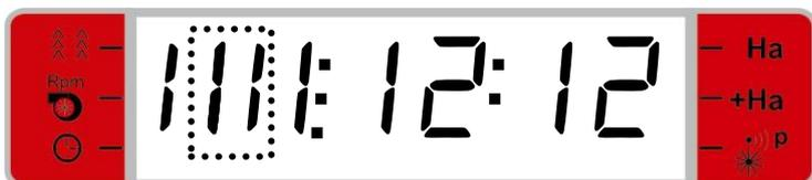
The display shows that a symmetric tramline is being laid in cycle 12. The symbol is flashing as a tramline is being laid in the “last” passage.
