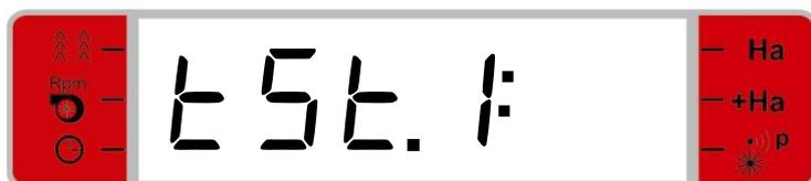
Display for test of keys (indicating "St. 1:" in the display)
