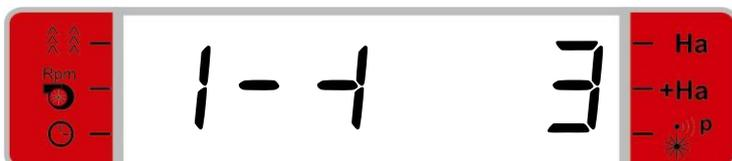
Setup of seeding width, here a 3 m seeder
