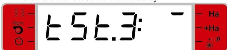
Activated cell pulse sensor is indicated by:
