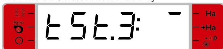
Activated cell pulse sensor is indicated by:
