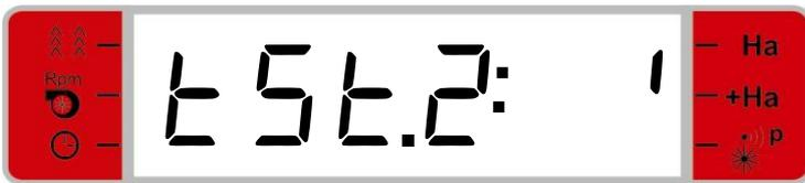
Example of test of
