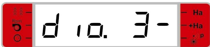
Display for test of LEDs. Here LED 3 is deactivated.
