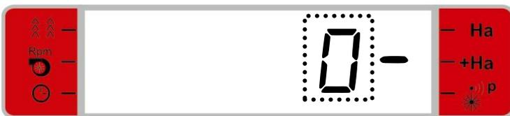
If you press the SET key for two seconds, this will imply that the reset total area is saved. If you do not want to reset the total area, you may press the EXIT key in order to maintain the previous value, and then the Controller will leave the edit mode and show the previous display. If you press the EXIT key again, the Controller will show the display for the tramline positioning.
