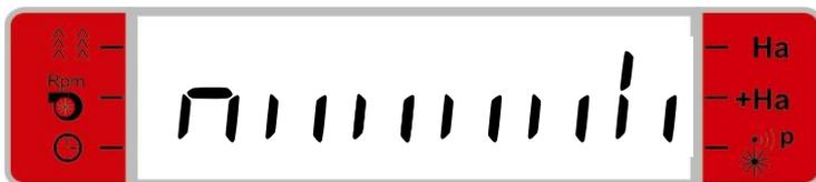
Asymmetric positioning with the actuator installed at the right side (top vertical *single* marking *to the right*) with full seeding width in the first passage (all the bottom vertical markings are activated) and with start in the left side (the horizontal marking in the left side). Correspondingly there is a display for actuator in the left side and with start in the right side.
