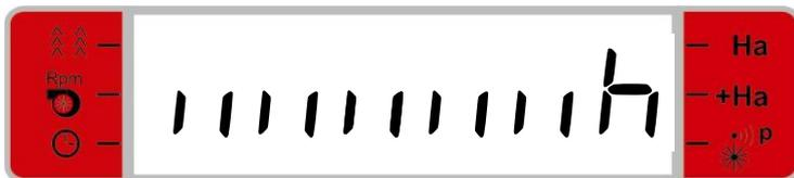
The above display shows asymmetric positioning (upper vertical *single* marking *to the right* of the display) with full seeding width in the first passage (all the bottom vertical markings are activated) and with the actuator installed in the right side and with start in the right side (the horizontal marking in the right side).
