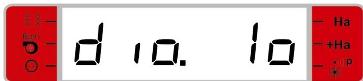
Display for test of LEDs. Here LED 1 is activated.
