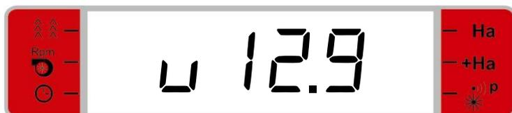
The display shows the current power supply. In this case 12.9 volt.
