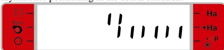
The above display shows symmetric positioning (upper vertical *double* marking in the *middle* of the display) with half seeding width in the first passage (only the right half of the bottom markings is marked). The start direction is optional.
