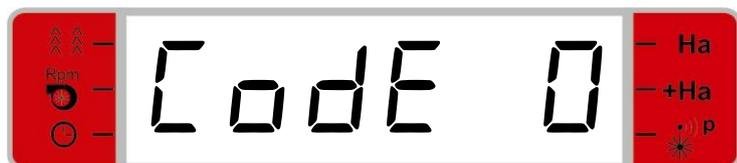
As the start-up passage has code 0, this display is established by pressing the SET-key.
