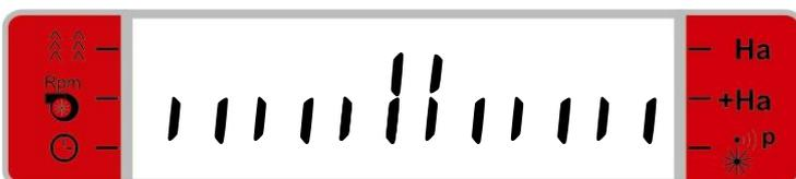
Symmetric positioning with full seeding width in the first passage. It is not possible to select asymmetric positioning.
