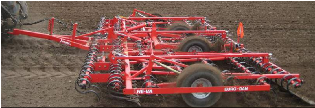
EURO-Dan Eco 8,00m w/Strong front-harrow, Spring-Boardspring tine levelling bar and Spring-Board after-harrow.
