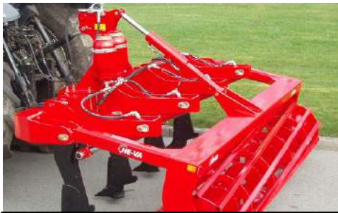
3,00 m w/hydraulic auto-release system, 4 tines, Square tube roller & hydr. depth control.
