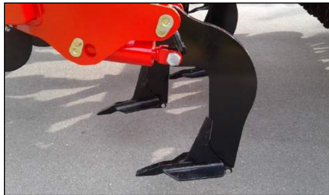
Tine design in Combi-Tiller MKII and Combi-Disc.
