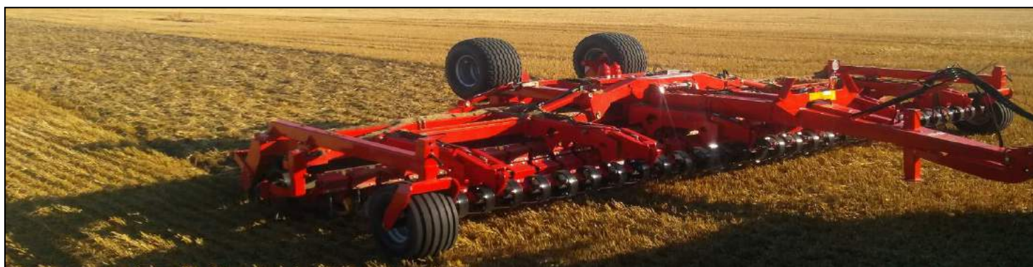
6.50 m Disc-Roller Contour w/V-Profile roller, material-damper guard, pivoting support wheels and two point pivoting crossbar.
