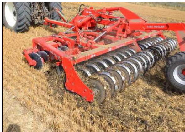
5.50 m Disc-Roller Contour w/Twin V-Profile roller and material-damper guard.
