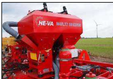
Multi-Seeder Twin 2x100-8-HY-AC - 593 x 926 (1180) mm H=935 (1075) mm
