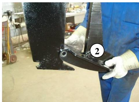
1.  $\triangle$  Before working with the machine's wearing points, the machine is to be fastened. This can be performed by trestles under the main frame or by a support of the roller.
