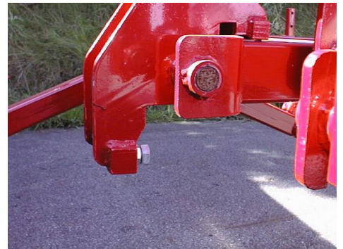
Adjustable stop for side frames.
