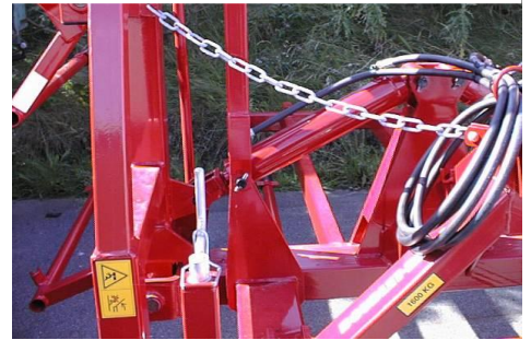
Security chain for side frames.
