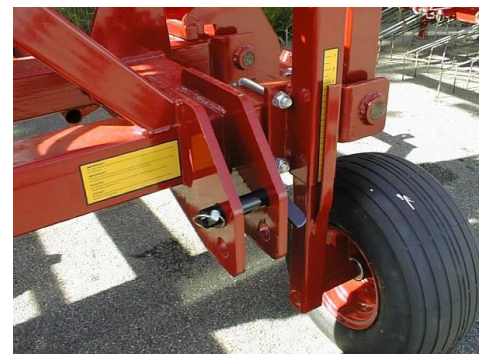
Attachment plates on 9,0 and 12,0 m.
