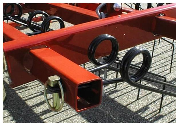
The tines are easily dismounted/mounted by means of a ring split.
