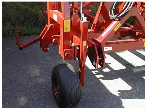
The support wheels have to be adjusted, so that the harrow frames are horizontal during work. Remember to lock the spindle.
