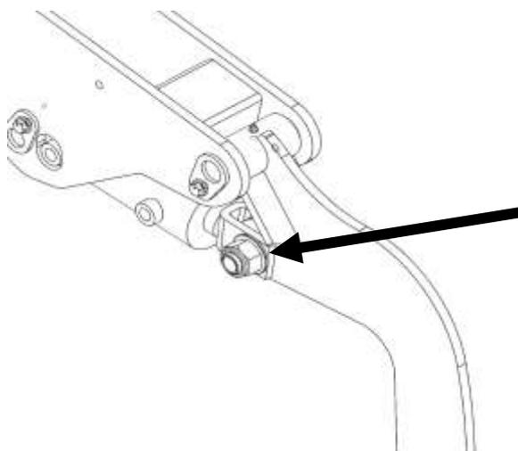
**Important to tighten up this bolt after 25 hours of operation when tine or cylinder has been replaced to 1000 Nm. When taking apart also check the bushing no. 645000113 for wearing.**
