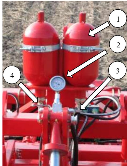
Before each season it has to be controlled, that the gas pressure in the accumulator (Pos.1) is 110 bars. **⚠** This requires special tools and can only be performed by an authorized dealer.
