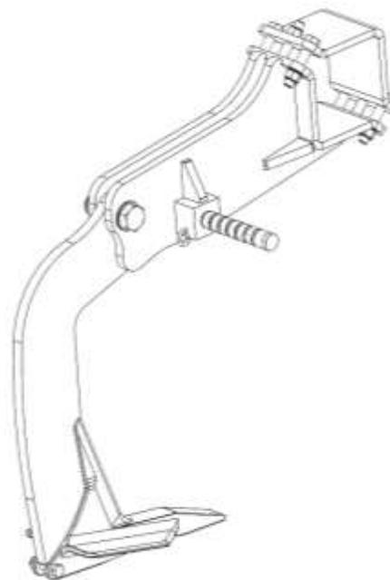
**Tine hydraulic with 200 mm wearing point, long model, (short not shown)**
