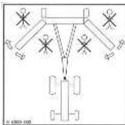
Always make sure that the working area of the wing sections is free before they are unfolded into working position.
