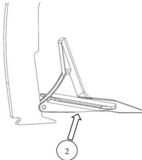
Mount the new wearing point, item no. 645000044 (Pos. 2), by pushing the wearing point to the rear and then in its place.
