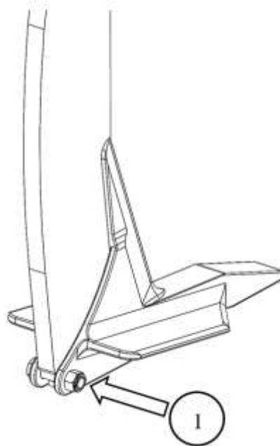
⚠ Before working with the machine's wearing points, the machine is to be fastened. This can be performed by trestles under the main frame. Dismount M16x65 mm bolt (Pos. 1) by means of 2 pcs. 24 mm spanners. ⚠ The wearing point might fall off, when the bolt is removed – **take care of foot and leg injuries.**
