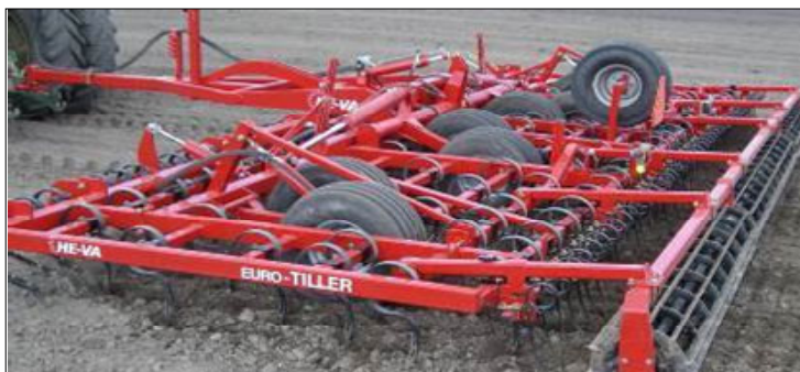
8,00 m Euro-Tiller w/ Spring-Board levelling bar, Flat bar roller incl. long finger after-harrow and spare wheel.
