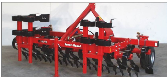
4,00 m Front-Board w/ slicing plates.
