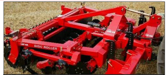
3,00 m three-point hitched Combi-Tiller MKI with 3,00 m three-point hitched Disc-Roller Contour .
