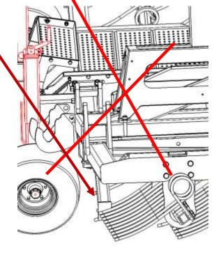
Tines at workingposition, when folding / unfolding
