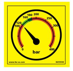
Correct hydraulic pressure on the release system.
