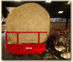
A unique feature on the machine are the twin-tined bale spears. The bale spears load the round bale onto the feeding platform. Without the driver or user of machine needs to leave the tractor seat, the bale spears can be docked into the feeder platform. Hereby the integrated hydraulic motor is automatically attached and the machine is ready for both transport and unwinding of bale material.
