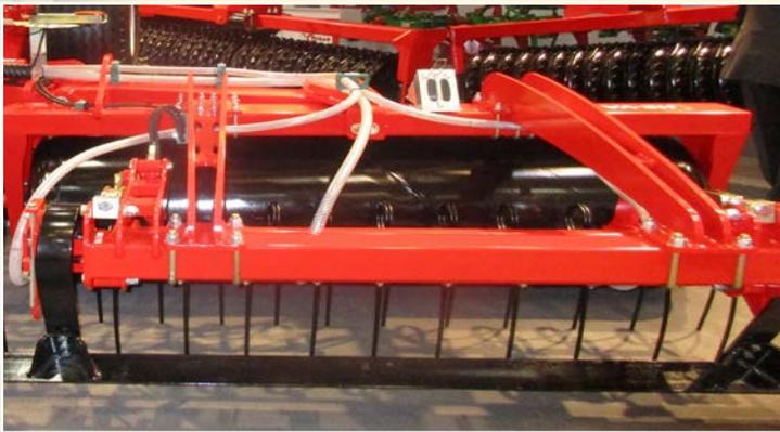
For intensive levelling of grassfields, an optional levelling board can be fitted on 2- and 4-row models and is fully adjustable.
