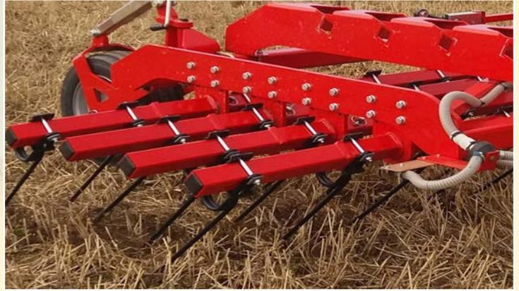
After harvest, the Top-Strigle spreads the left-over straw and by lying straw to sunlight, the germination process will be accelerated. This creates optimum conditions for direct drilling.
