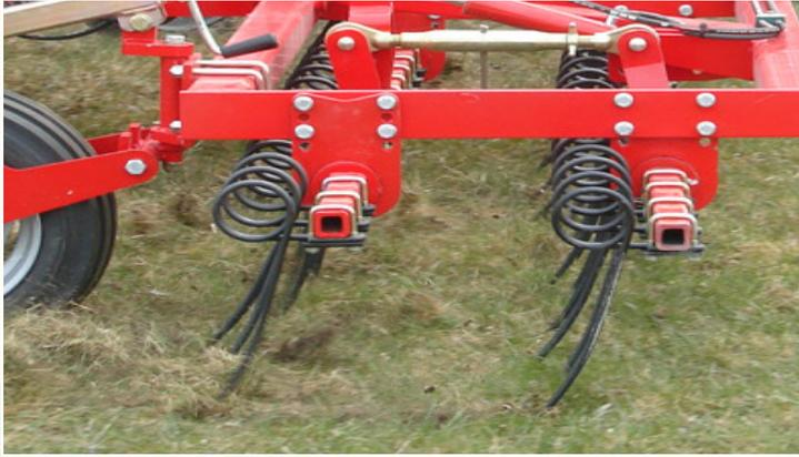
The Top-Strigle freshens up the field after the winter season, where it levels and breaks up the surface to allow oxygen to get to the root zone and helps to create tilth to make the seed germinate.
