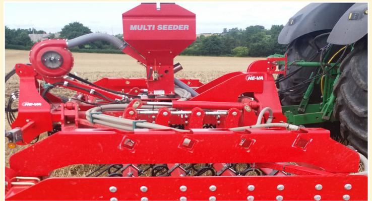
Combine the Top-Strigle with a Multi-Seeder and be able to do direct tilling at the same time as creating a quick and effective germination of weed seed.
