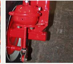
Wheel set making an attachment of rollers possible behind a harrow. Wheels: 11.5/80 x 15.3
