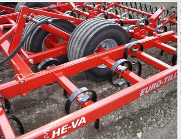
The strong 10 x 45 mm harrow tines ensure an optimal harrowing of all soil types.
