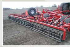
A flat bar roller Ø400 mm mounted with the longfinger harrow in front leaves a pulverized and light consolidated surface. With its construction of 8 x 40 mm flat steel, this type of roller ensures a perfect soil structure.
