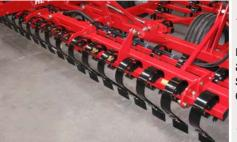
By mounting a Spring-Board in front of the Euro-Tiller, the field is perfectly levelled and the major clods are broken. The Spring-Board tine is a strong  $10 \times 80$  mm spring tine, standard mounted with  $8 \times 150$
