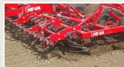
With the front harrow mounted before the front Spring-Board, the crust and wheel tracks or compressed soil is loosened so that the levelling bar performs a more precise levelling of the already loosened soil with a
