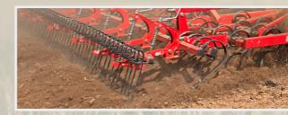
The solid longfinger afterharrow mounted with strong 12 mm back bended tines never leaves anything in bulks and it erases the harrow tine tracks effectively.
