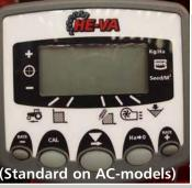
The seed rate is set by the Auto-Controller and the seed rate can be adjusted by the control box in optional steps. The calibration can be set when activating the dosage unit by pressing the el-switch on the Multi-Seeder. Auto-Controller has surveillance and alarm functions for fan operation and low seed hopper level as well as a prestart function for start of seeding in the field edges etc. Finger switch (top link) for start and stop of seeding is included.
