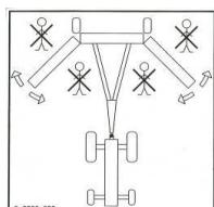
Take care that no persons are within the machine's hazardous area during the unfolding and folding procedure.
