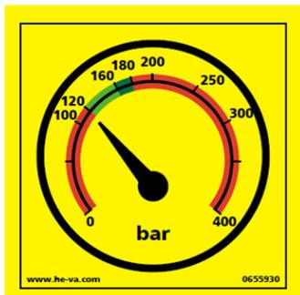
Correct hydraulic pressure on the release system.
