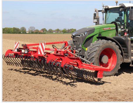
3.00 m Front-Roller Twin with Ø550/550 mm Star rings
