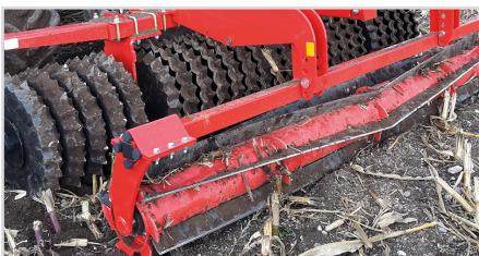
Top-Cutter on Front-Roller
