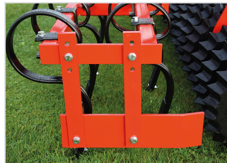
Edge equipment set for front harrow
