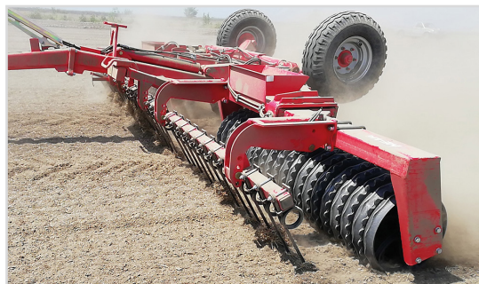
6.30 m Tip-Roller with Cambridge rings and Spring-Board with Ø16 mm longfinger tines
