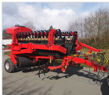
Folded Tip-Roller with Multi-Seeder, Spring-Board and wheel track eradicator
