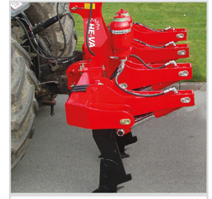
3.00 m. with hydraulic auto-release system and 4 tines.
