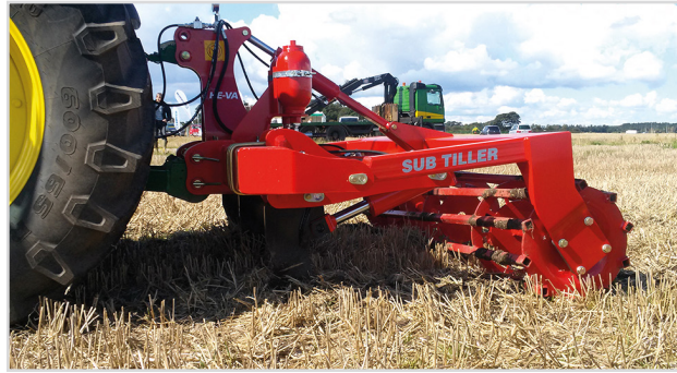
3.00 m. with hydraulic auto-release system and 4 tines.
