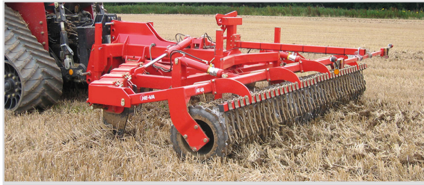
5.00 m Sub-Tiller with V-profile rings and hydraulic automatic stone protection
